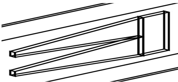
Figure 2: The eRHIC synchrotron radiation absorber.
