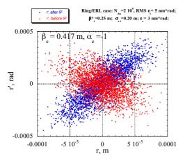
Fig. 2. Round 10 GeV electron beam from ERL with initial transverse RMS emittance of 3 nm rad passes through the IP with the disruption parameter 3.61 (tune shift  $\xi_{xe} = 0.6$ ). The emittance growth is only 11%.
