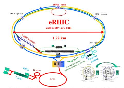
Fig.1. Main layout of ERL based eRHIC with up to four IPs and possible 5 GeV polarized positron storage ring. Polarized electrons are generated at a strained GaAS photocathode, accelerated in a multi-pass ERL, used in one –to-four collisions with the hadrons contra-rotating in the RHIC blue ring, decelerated and finally dumped.
