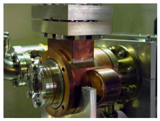
Figure 1: The 2856 MHz microwave gun cavity fabricated in house at NSRRC.
