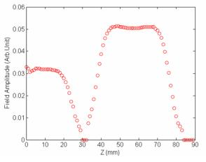
Figure 6: Measured electric field amplitudes (arbitrary unit) as a function longitudinal position. The position zero is the location of the thermionic cathode.
