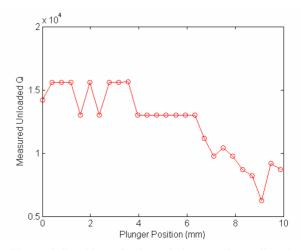
Figure 5: De-Qing of  $\pi/2$ -mode by coupling cell tuning.
