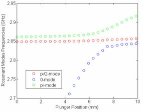
Figure 3: Dependence of eigenmode frequencies on sidecoupled cell tuning plunger positions.
