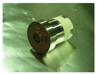
Figure 2: Thermionic cathode (with nose cone) assembly purchased from HeatWave Labs, Inc.
