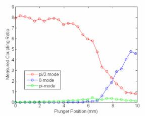
Figure 4: Measured coupling coefficients of the resonant modes versus plunger positions.
