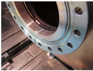
Figure 7. Port flange e-beam welded to cavity.
