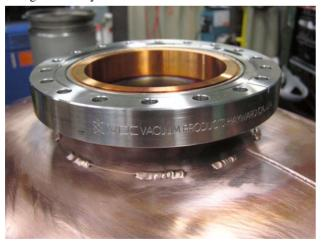
Figure 8. Port repaired by TIG welding.
