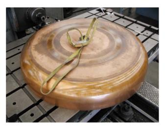
Figure 1: Spun cavity half-shell.
