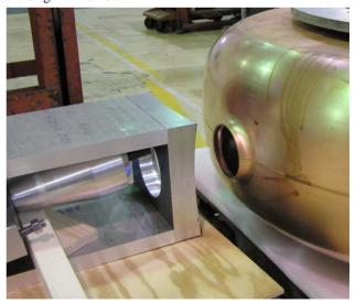
Figure 6. Port pulling after e-beam annealing.
