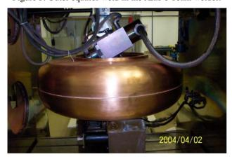
Figure 4. Inside cosmetic weld in the JLab e-beam welder.
