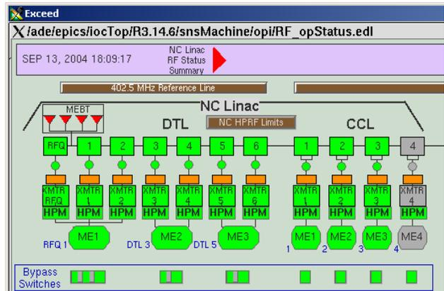
Figure 4: Normal Conducting Linac portion of the Status Screen in EPICS.
