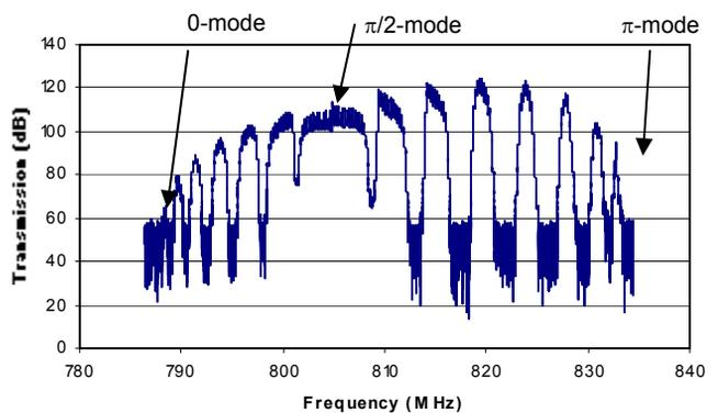
Figure 2: Measured mode spectrum in CCL Module 1 after tuning.
