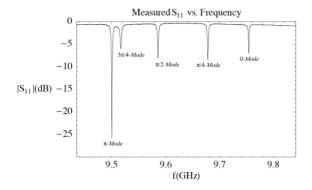
Figure 5: Plot of the RF reflectance at the input coupler of the prototype cavity showing the 5 non-suppressed resonances.
