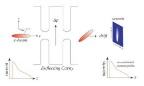
Figure 2: Illustration of the deflection of a beam by a dipole mode cavity phased at the zero-crossing of the RF.
