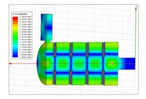
Figure 3: Plot of deflecting mode cavity geometry (quarter view) and axial transverse magnetic field profile from the center cell to the exit of the structure from HFSS simulations (quarter view).
