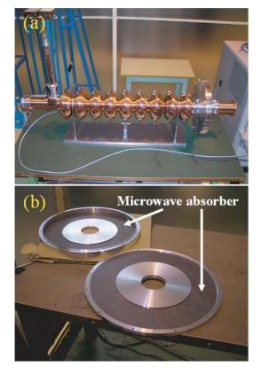
Figure 2: (a) A low-power model of 9-cell TESLA-type cavity with a radial-line HOM damper. (b) Inside of the radial-line HOM damper.
