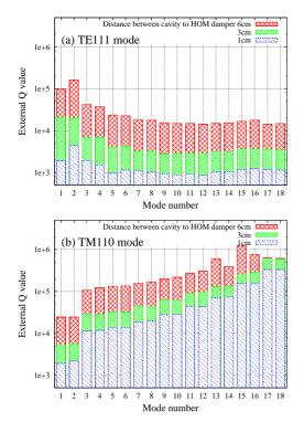
Figure 5: Measured  $Q_{\text{ext}}$  for the (a) TE111 and (b)TM110 modes. The red, green and blue bars indicate the results under the conditions of (2), (3), and (4), respectively.
