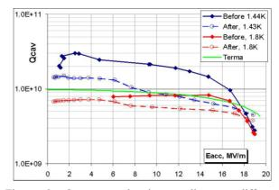
Figure 9: Q vs. accelerating gradient at different temperatures
