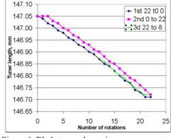
Figure 6: Blade tuner elongation measurement
