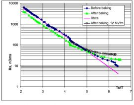
Figure 8: Resistance vs. Temperature
