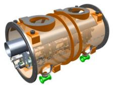
Figure 1: Cryomodule design for 4 cavities.
