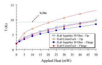
Figure 6. Flange and probe tip temperatures as a function of heat applied to the probe tip, two designs.
