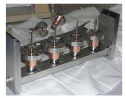
Figure 4. JLab single-crystal sapphire RF feedthroughs.
