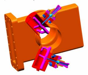
Figure 1. Cross-section of two HOM couplers between the FPC and cells of the HG and LL cavities.
