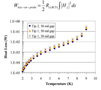
Figure 3. Heat load on Nb probe in HG & LL cavity HOM coupler at 20 MV/m CW, assuming Nb BCS surface impedance at 1.5 GHz.
