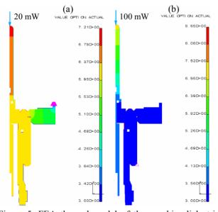
Figure 5. FEA thermal model of the sapphire-dielectric RF feedthrough with a) 20 mW load to tip and 3 K flange, and b) 100 mW load to the tip with 3 K copper collar. In both cases, the probe tip stabilizes at 6.9 K.
