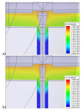
Figure 2 The local magnetic field around probe Tip 1 (a), and Tip 2(b).
