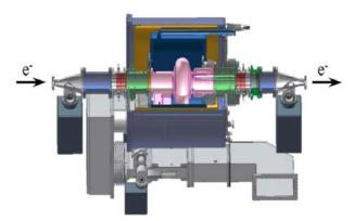
Figure 1: CESR-type cryomodule for TLS.
