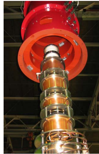
Figure 5: Klystron assembly prior to full power tests.
