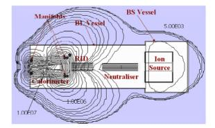
Fig. 4: Neutron flux  $(n/cm^2s)$  for an average current of 1 A.
