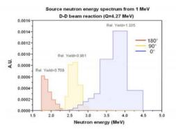
Fig. 1: D-D neutron spectrum.
