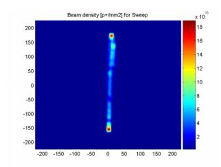
Figure 3: Sweep profile  $(p+/mm^2)$  at TDE entrance window, for all MKBH missing (450 GeV ultimate beam).
