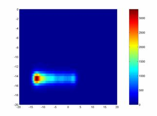
Figure 7:  $\Delta T$  for total dilution failure on a 200  $\mu$ m stainless steel foil, after 15 mm of CC (7 TeV ultimate beam).
