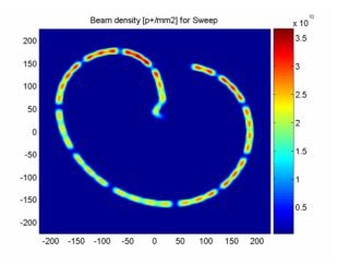
Figure 2: Nominal sweep profile (p+ / mm<sup>2</sup>) at TDE entrance window (450 GeV ultimate beam).
