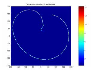
Figure 6:  $\Delta T$  for nominal sweep on 15 mm of CC (7 TeV ultimate beam).
