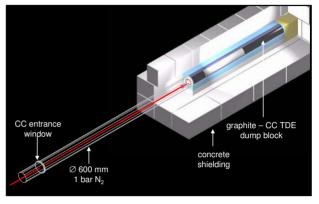
Figure 1: LHC dump block TDE and surrounding shielding, showing location of entrance window.
