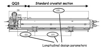
Figure 1: Main cryostat design parameters for an SSS
