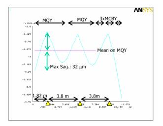
Figure 2: Calculated deflections for Q4 & Q5 in IR2 & 8.
