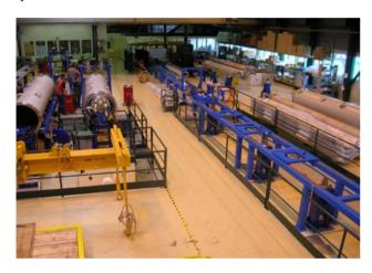
Figure 5: MS SSS Assembly benches: SSS with 2 supports (left), SSS with 3 supports (right).
