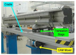
Figure 1: Prototype precision positioning system for the LCLS undulators.
