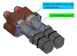
Figure 2: Double cam-shaft mover assembly.
