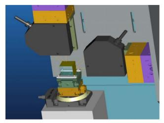
Figure 3: Reference surface and laser displacement sensor setup at the end of the cradle.
