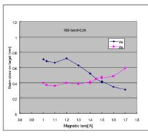
Figure 9a: Beam sizes versus magnetic-field strength.
