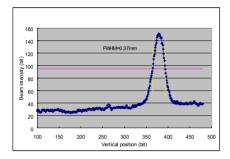
Figure 8b: Vertical cross section of a beam spot observed by a pinhole camera.
