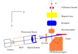
Figure 1: System configuration of main components. An electron beam is focused on a target after being bended by 180 degrees. A pinhole camera measures the beam size on the target.
