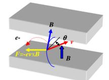
Figure 2: Relation between an injection angle  $\theta$  and a vertical focusing force produced by a fringing field **B**.
