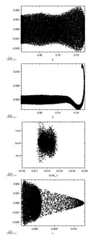
Figure 4: Beam trajectory simulation from an electron gun to the target.
