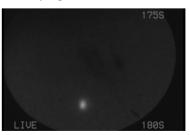
Figure 7b: Typical beam spot observed by a pinhole camera.
