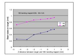
Figure 9d: Beam-sizes measured in the region near the target. The beam is vertically defocused. ( $\theta < 0$ )
