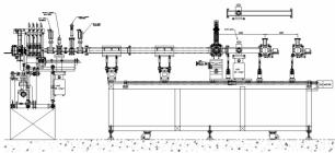
Figure 4. The left side part is the RF PC gun assembly with RF PC gun, solenoid, Laser incident chamber, and beam diagnostic chamber. The right side part is the Emittance-Meter with the bellows, pin-hole plate chamber, and YAG screen chamber.
