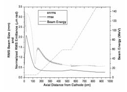
Figure 2. The beam size, emittance, and energy of our beam along the RF PC gun with the solenoid field profile is simulated by PARMELA code.
