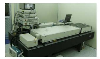
Figure 3. Ti:Sapphire laser system with 267nm wavelength is installed.
