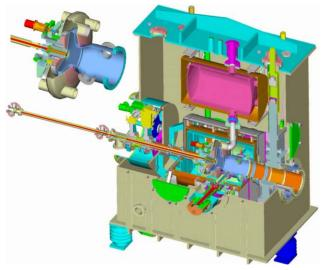
Figure 6: SRF gun cryostat and cavity detail (upper left).
