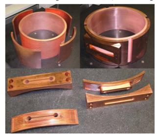
Figure 5: NCRF gun cell 2 (upper left) and cell 3 (upper right) plated and ready for brazing. Waveguide irises machined and ready for plating (lower).
