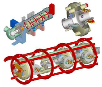
Figure 1: DC Gun and SRF booster (upper left) showing 3<sup>rd</sup> harmonic (lower) and fundamental cavity (upper right).
