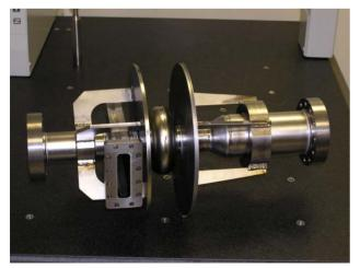
Figure 3: 2245.5 MHz third harmonic SRF cavity.
