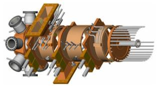
Figure 4: Normal-conducting 2<sup>1</sup>/<sub>2</sub>-cell CW RF gun.
