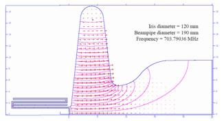
Figure 7: SRF gun choke joint and <sup>1</sup>/<sub>2</sub> cell cavity.
