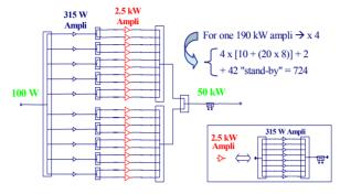
Figure 7: Power combination scheme (50 kW "tower").
