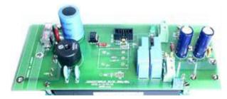
Figure 2: DC/DC converter board.
