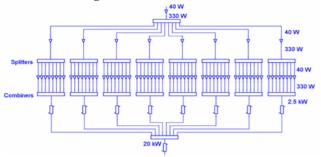
Figure 3: Power combination (1/2 BO amplifier).
