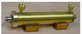
Figure 5: Coaxial measuring line for coolants.
