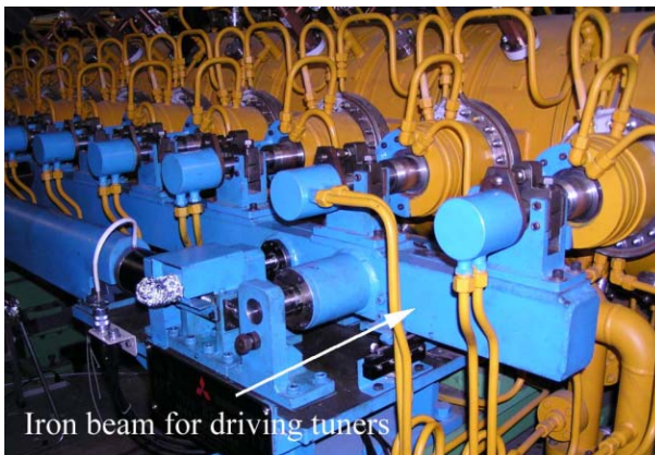
Figure 6: Common driving mechanism for the tuning plungers of the APS cavity.
