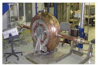
Fig. 3, The 201 MHz Cavity.
