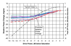
Figure 4: Relative Phase Change vs. Drive Power
