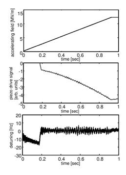
Figure 6: Top: Cavity filling at  $Q_L = 1.2 \cdot 10^8$ . Middle: Piezo drive signal during the same time period. Bottom: Cavity detuning during the same time period.
