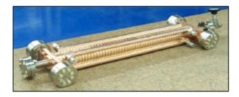
Figure 4: A 60cm NLCTA Accelerating Structure.
