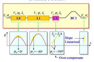
Figure 1: Schematic of two linac segments followed by harmonic RF and compressor chicane. The bunch is compressed from an initial rms length  $\sigma_{z0}$  to a final length  $\sigma_z$  with initial energy  $E_i$  and final energy  $E_0$  (bunch head at left: z<0).
