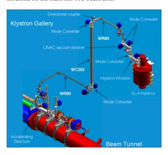
Figure 2: LCLS X-Band RF System Layout.
