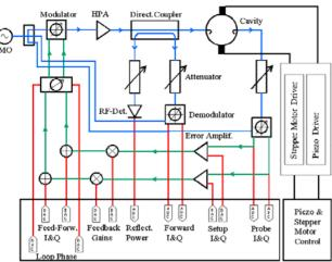
Figure 1: Low Level RF block-diagram.
