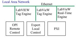
Figure 3: Low Level RF communication network and software interface.
