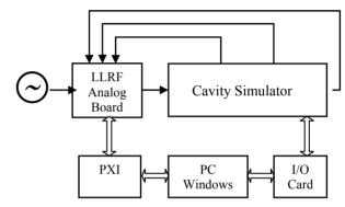
Figure 5: Block diagram of Low Level RF test assembly.
