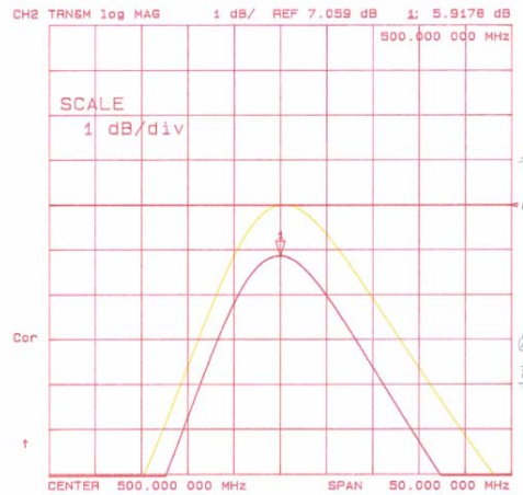
Figure 9: Resonant combiner with 4 active inputs and the 5 th connected to chosen impedance.
