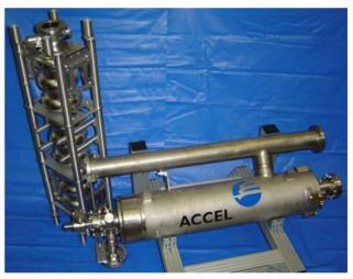
Figure 7: TESLA cavity for BESSY furnished with helium vessel, HOM couplers and input coupler. The cavity is prepared for cold horizontal RF Test in the HoBiCaT cryostat. The second cavity installed into the transport frame is shown in the left.
