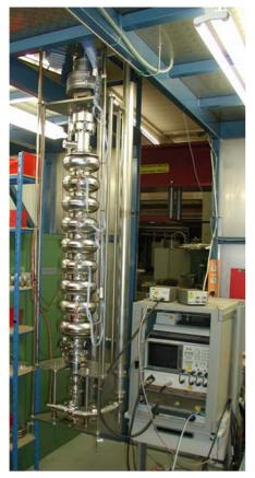
Figure 2: TESLA cavity assembled to the vertical test stand at DESY
