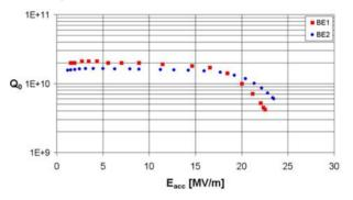
Figure 4: Test results of cavity BE1 and BE2. Fields above 20 MV/m with Q higher than  $1 \cdot 10^{10}$  were reached. At the highest fields some field emission was observed. Both cavities were checked for Q-disease and proven to be Q-disease free.
