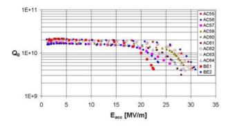
Figure 5: Comparison of cavities prepared at ACCEL for BESSY and cavities prepared by DESY (published in the TESLA TDR). BESSY cavities received 800 °C heat treatment, DESY cavities received 800 °C and some additional 1400 °C heat treatment.
