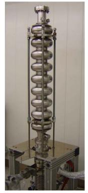
Figure 1: TESLA cavity during high pressure water rinsing at ACCEL. The high pressure water rinsing system is installed in a class 100 clean room.
