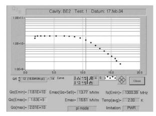
Figure 3: First test of cavity BE2. Field emission limited the cavity to about 16.8 MV/m.
