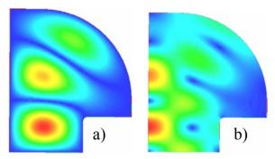
Figure 1: Geometry of our test cavity and false-color plots of the a) E and b) H field patterns for the  $TE_{013}$ -like mode. The left edge is the symmetry axis, and the bottom edge is the face of the test sample.
