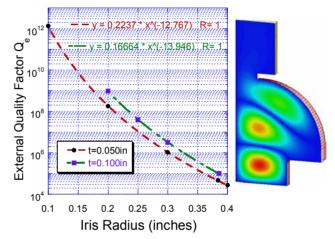
Figure 3: Dependence of the external quality factor,  $Q_e = \omega U/P_e$ , on the iris radius, with two iris thicknesses. Also shown is the final geometry for copper.
