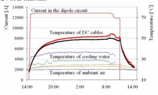
Figure 1: Current in the warm circuits and temperatures during a typical 24-hour heat run of the converters in one of the LHC powering areas.
