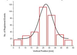
Figure 3: Beam profile measured at  $10^{-7}$  mbar pressure in the COSY ring (Gaussian fit to channel data). Events have been summed up for 4 seconds. Beam data: 1 GeV, ~5•10<sup>9</sup> protons.
