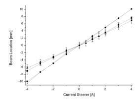
Figure 4: Beam position versus steerer strength measured with our optical beam profile monitor ( $\blacktriangle$  and  $\blacksquare$ ) and a BPM ( $\bullet$ ) located downstream.
