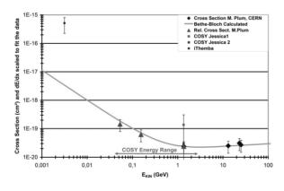
Figure 6: Cross section for light production for  $N_2$ versus proton energy. The graph shown is based on the Bethe Bloch formula fitted to reference values from [9].
