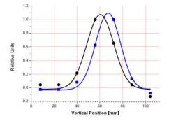
Figure 2: Singe pass beam profile of a pulsed (1.35 GeV, p=10 mbar) normal positioned (•) and shifted (•) beam (Gaussian fit to PMT data).
