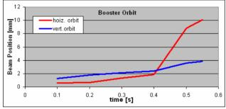
Figure 5: Horizontal and vertical orbit in the booster. The large jump after 0.4 s is due to the excitation of the bumper magnets for the extraction.
