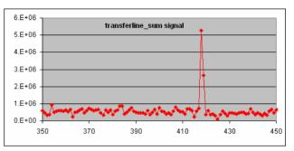
Figure 1: Sum signal from a BPM in the Booster to Storage ring transfer line. The bunch train is 70 ns long. The turn by turn spreads it over 2 turns (736 ns).
