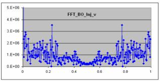
Figure 3: FFT of the vertical Booster orbit at Injection.
