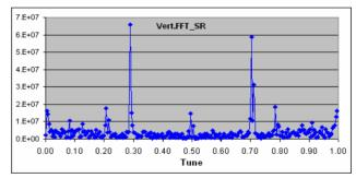
Figure 9: FFT Spectra of the vertical beam position.
