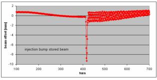
Figure 13: Orbit bump induced by the Septum and the Kickers in the injection section.
