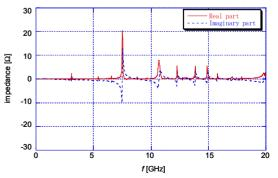
Figure 4: Longitudinal impedance spectrum of asymmetric BPM for KEKB HER. The solid and dotted lines are the real and imaginary parts, respectively.
