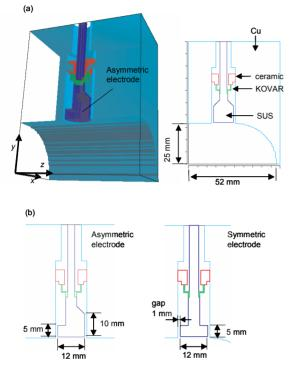
Figure 1: BPM for KEKB HER. (a) 3D cut model of asymmetric electrode and its cross-section (x-y plane). (b) Cross-section of the asymmetric and symmetric electrode (y-z plane).
