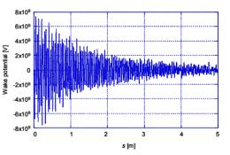
Figure 3: Longitudinal wake potential of asymmetric BPM for KEKB HER.
