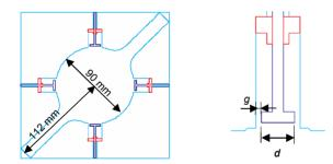
Figure 2: Cross-section of a beam duct with antechambers with BPMs for SuperKEKB modelled by MAFIA.
