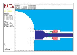
Figure 5: y component of magnetic field of the TE110 mode calculated by the Eigenmode solver.
