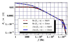
Figure 1: Longitudinal impedance for the case of a (single-layer) 1 m long (round) LHC graphite collimator with radius b = 2 mm and conductivity  $\sigma = 10^{-5} \Omega^{-1} \text{m}^{-1}$ .
