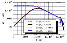
Figure 2: Transverse impedance for the case of a LHC graphite collimator (see Fig. 1).
