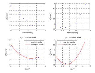
Figure 6: Measured horizontal and vertical emittance of the 50 MeV lianc by quadrupole scan method. The fitted normized emittance is  $\varepsilon_x = 1.09$  mm-mrad and
