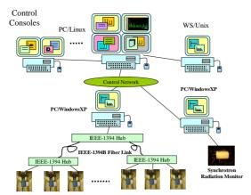
Figure 1: Topology of the IEEE-1394 camera installation.
