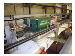
Figure 4: The first chicane magnet and BPM5 in the ESA beamline.
