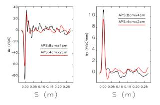
Figure 1: Total wake potentials of the APS storage ring excited by the 5-mm bunched beam. The one in the current vacuum chamber in black is compared to the one in the proposed small chamber in red curve: Wz (left) and Wy (right), respectively.
