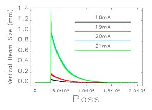
Figure 3: The vertical beam size variation of the bunched beam kicked in the vertical plane by 0.1 mm at turn 3000.
