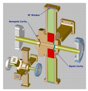
Figure 2: X-band cavity BPM cross section.
