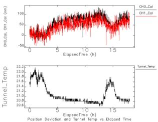
Figure 3: Electronics thermal stability test.
