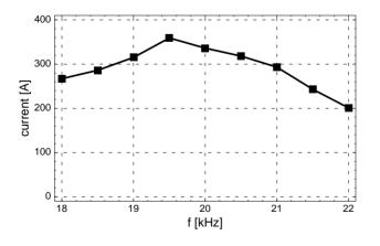
Figure 5: The maximum produced current vs frequency.
