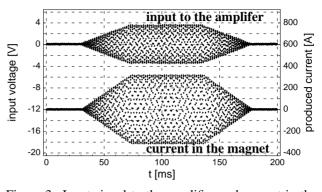
Figure 3: Input signal to the amplifier and current in the magnet. The input is created by two waveform generators. One creates 20 kHz sine waves and the other modulate its amplitude. The signal noise ratio of the current in the magnet was more than 20 dB in this case.
