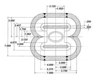
Figure 2: Design drawing of the Tevatron vertical AC dipole magnet. Dimensions are given in inches.
