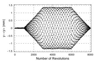
Figure 6: Turn-by-turn positions of the oscillations excited by the Tevatron vertical AC dipole.
