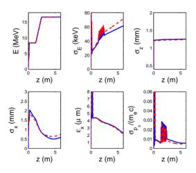
Figure 2: Comparison of beam parameters obtained with ASTRA (blue solid line) and IMPACT-T (red dashed line) when space charge effects are included. The parameters are: E is the energy of the beam,  $\sigma_E$  is the rms energy spread,  $\sigma_z$  is the bunch length,  $\sigma_x$  is the beam spot size on the cathode,  $\epsilon_x$  and  $\sigma_{px}$  are respectively the rms transverse emittance and momentum spread.
