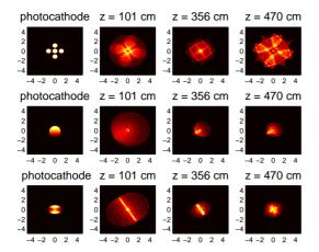
Figure 3: Transverse beam distributions at different locations along the AWA obtained by tracking an initial quincunx distribution (top row), dipole (middle row) and quadrupole (bottom row) perturbations.
