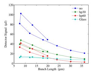
Figure 7: Bunch length sensitivity for the BC2 bunch length monitor. The "Glass" curve is for a 3 mm thick fused silica plate as low pass filter at 30 cm<sup>-1</sup>.
