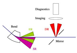
Figure 2: Schematic of the different radiation sources from a bend magnet. The synchrotron (SR) and the edge (ER) radiation are coupled into a detector with a hole mirror, which itself generates diffraction radiation (DR).
