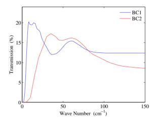
Figure 4: Simulated transmission spectrum of edge radiation in percent of the ideal far field intensity after passing through the bunch length monitor setup designed for a downstream location after bunch compressor 1 (BC1) and 2 (BC2).
