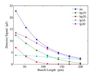
Figure 6: Bunch length sensitivity for the BC1 bunch length monitor. The detector signal represents the effectively deposited energy in a  $100 \, \mu \text{m}$  thick LiTaO<sub>3</sub> pyroelectric detector element for different frequency filters where "lp" means low pass and "hp" high pass. The subsequent number is the cut-off wave number in cm<sup>-1</sup>.
