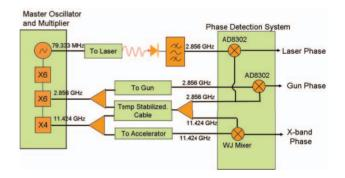
Figure 1: Schematic of the RF phase detection system implimented at the NLC Test Accelerator at SLAC.
