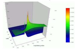
Figure 6: Electric field distribution at an open corner of a tile
