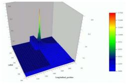
Figure 4: Electric field distribution in the region between an omega seal and ceramic tiles.
