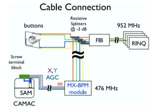
Figure 1: Test setup used in LER of PEP II. The upper path describes the original PEP II BPM installation. Before the the FIB the signal is split and half of the signal is brought to the BERGOZ module. The position analog output is digitized by the SAM and included in the SCP as Analog STatuS (ASTS) channel.
