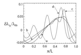
Figure 1: An initial sinusoidal perturbation with  $\eta_{b0}^{max} = \delta \lambda_b^{max}/\lambda_{b0} = 0.05$  and  $v_{b2}r_w/v_{b0}L = 10^{-2}$  (a) steepens due to the nonlinearity (b). A modulational instability at the back of the wavefront develops (c), and results in the formation of a train of solitons with different amplitudes (d).
