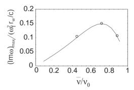
Figure 2: Plot of the normalized maximum growth rate  $(Im\omega)_{max}/(\omega_f^2 r_w/c)$  of the Weibel instability versus the average depressed tune  $\bar{\nu}/\nu_0$ .
