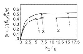
Figure 1: The normalized growth rate  $(Im\omega)/(\widehat{\omega}_{pb}v_{\perp b}^{th}/c)$  of the Weibel instability is plotted versus  $k_z r_b$ . Here,  $\widehat{\omega}_{pb}$  is the on-axis beam plasma frequency.
