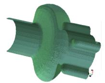
Figure 2: One-half of the CESR-B RF cavity. 3D GdfidL model.
