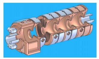
Figure 5: Cut-away illustration of the Positron Capture Cavity.
