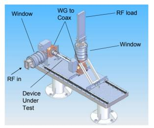
Figure 4: Illustration of the coupler component test stand.
