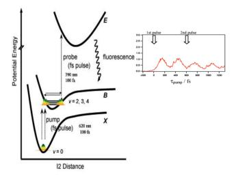
Figure 3: Pump-control-probe scheme for real-time measurement of wavepacket interference using fs pulses in the B-state of the  $I_2$  molecule [15]. The quantum interference is detected as oscillations in the fluorescence signal as a function of the time delay between the pump and probe pulses,  $\tau_{probe}$  (inset, right). Reproduced with permission of Kiyoshi Ueda.
