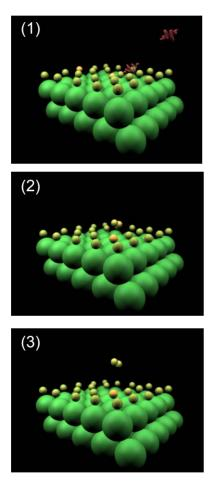
Figure 4: FEL-induced hydrogen desorption from a Si (111) surface. Si atoms are shown in green, and H in yellow. FEL photons come in and one photon excites one hydrogen adatom (1). Two excited neighbouring hydrogen adatoms pair up and as a result of "energy pooling" desorb associatively at room temperature (2) & (3). Figure reproduced with permission of N H Tolk [17].
