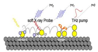
Figure 1: A pump-probe measurement at a surface. A very low energy terahertz (THz) pulse causes initial dissociation of a molecule (yellow) at a surface at time  $t_0$ . The reaction is followed at times  $t_1$  and  $t_2$  using synchronised soft X-ray photons (blue) that monitor the reaction of the dissociated atoms with new species to form the product. (Adapted from original figure by Anders Nilsson and colleagues at SLAC [5]).
