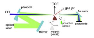
Figure 2: Schematic experimental arrangement for a gasphase pump-probe experiment using the FLASH facility at the DESY Laboratory in Hamburg in combination with an optical laser. 'One-shot' experiments are possible using time-of-flight (TOF) detection of the electrons produced. Adapted from reference [10] and reproduced with permission of M Meyer.
