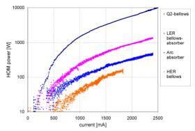
Figure 2: Measured HOM power in the PEP-II absorbers.
