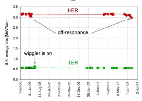
Figure 9: S.R. energy loss per turn.
